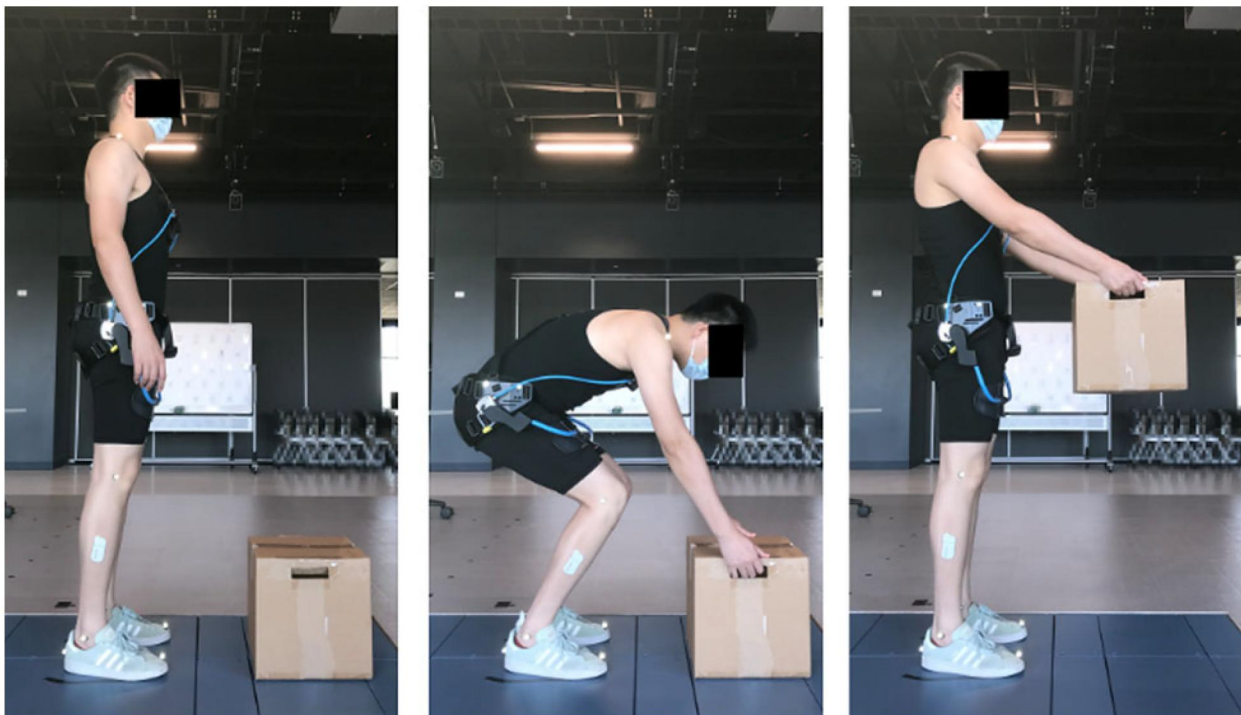
Figure 3. A subject performing the squat lifting task with the low-back exoskeleton. BioStamp sensors on the back were directly attached to the skin beneath the exoskeleton.
